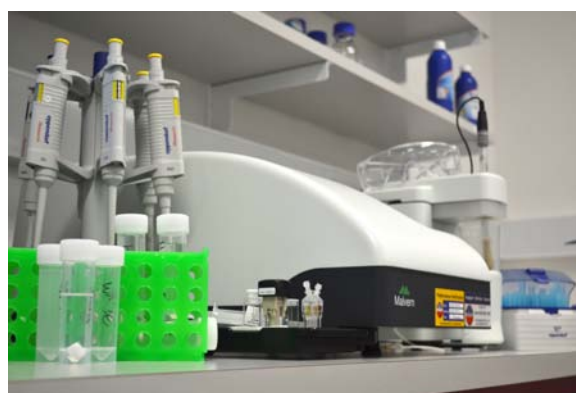
Above: The Malvern Zetasizer Nano ZS allows users to characterise a range of particles using minimal sample volume.
