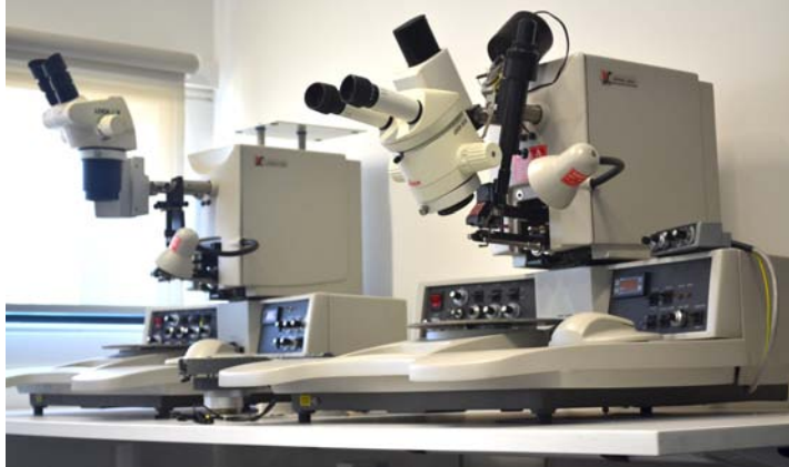
Above: The Kulicke & Soffa Ball and Wedge Bonders are available to all licensed users of the MCN
