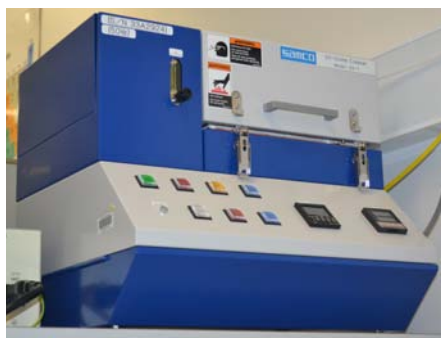
Above: The Ozone Cleaner, provides users with a non-chemical alternative for removing organic materials from surfaces.
