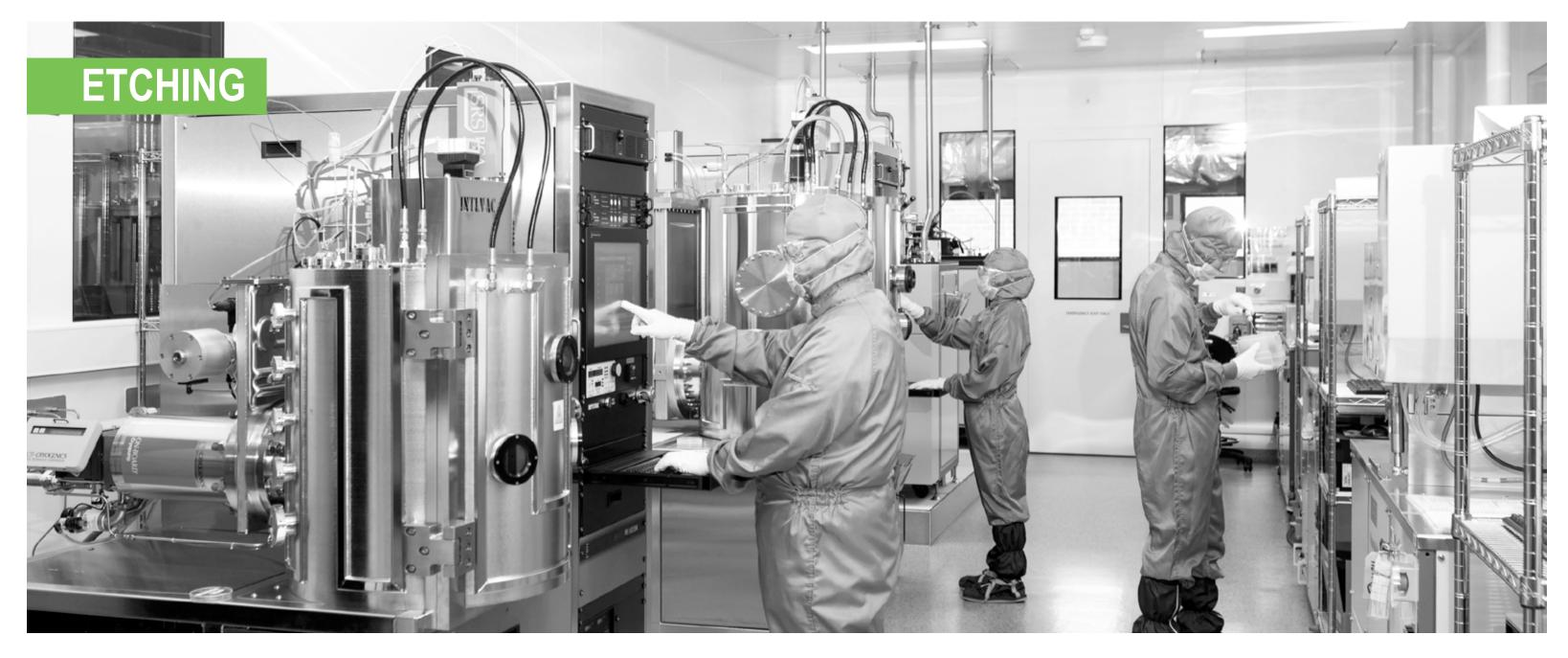
Reactive Ion Etching (RIE) combines chemical and physical etching to remove material deposited on wafers. Deep reactive-ion etching (DRIE) is a highly anisotropic etch process used to create high aspect ratio structures on substrates.
