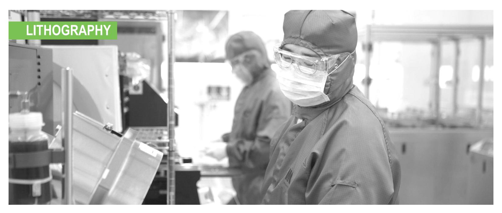
Micro-nano lithography is the process by which a pattern is written or transferred to a substrate. The process can be physical in nature, utilising a 'stamp' to press structures into a softer material, or chemical using light, ions or electron energy to write into photo and electron sensitive resists. This is necessary for the creation of the nanoscale components featured in nearly all modern technologies.
