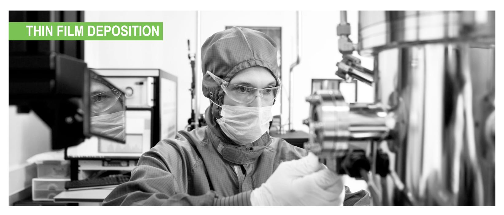
Thin film deposition is a process whereby materials - generally precious metals or oxides - are deposited onto a substrate or lithography sample. This can be achieved in a variety of ways such as sputtering, electroplating, evaporation, or CVD. MCN offers a range of different thin film deposition techniques and instruments, which are briefly explained here.
